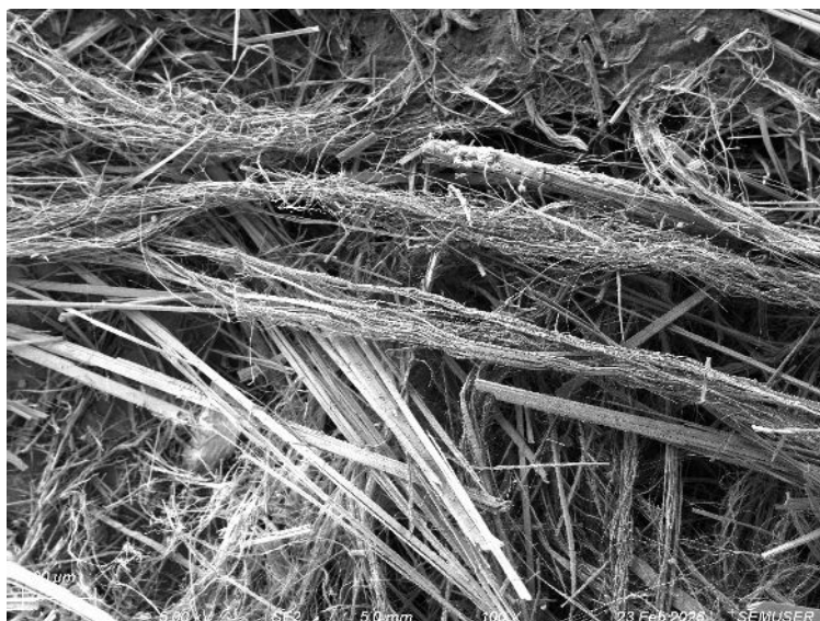
Figure 15: Frame-integrated SEM image collected using the SE2 detector at an accelerating voltage of 5kV, a working distance of 5.0mm, and a magnification of 100X.
