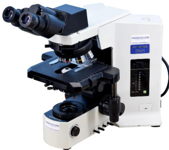
Figure 2: Olympus BX51 Light Microscope.
