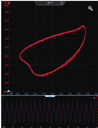
FIG. 3. Period-1 Behavior observed at 1.5V.
